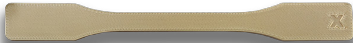
3d printed polymer part after the vibratory finishing process
